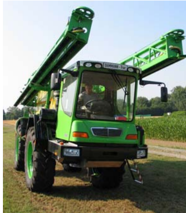
Fig.4: Right sprayer side with lateral folded boom and ascent to the drivers cabin.
